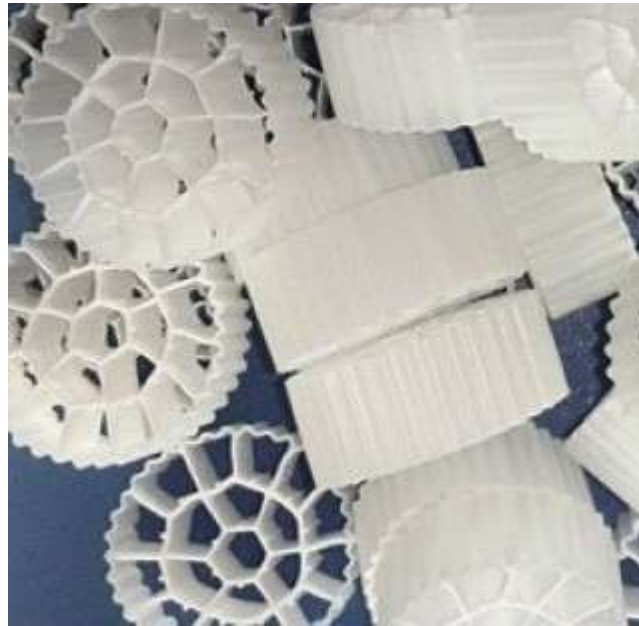
Figure 1. Typical MBBR media carriers [11]
