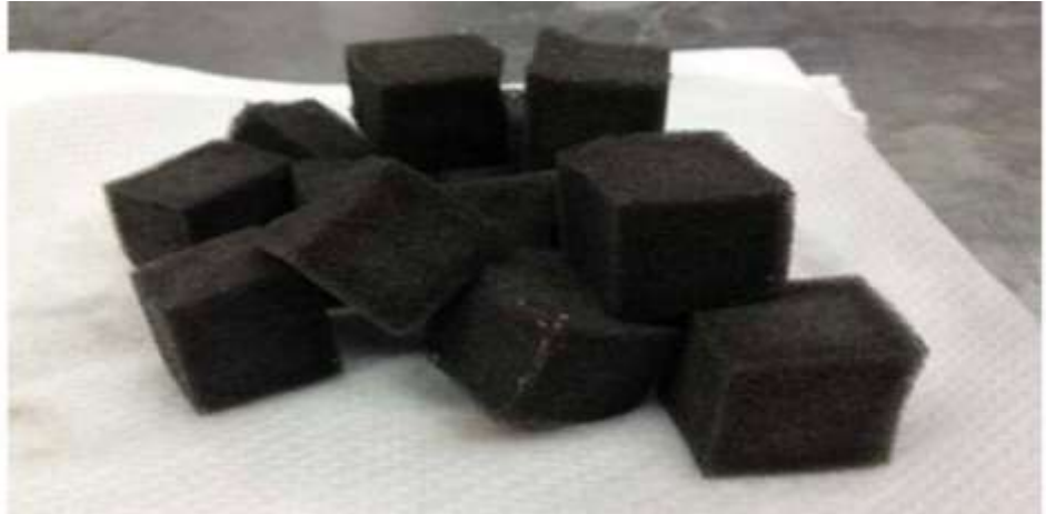
Figure 3. Cubes of Polyurethane sponge with attached-growth biomass
